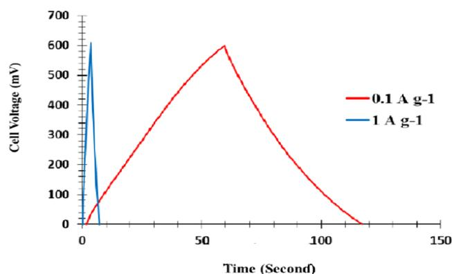
**Figure.6-** Charge discharge curves of GO/rGO composites at current density of 0.1, and 1 mA/cm<sup>2</sup> in a voltage range of 0 - 1000mV in a three-electrode system.
