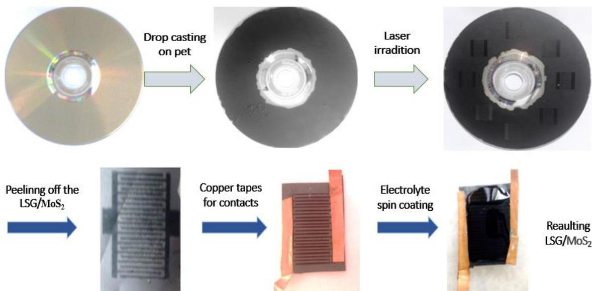
**Figure.1.** Schematic representation of flexible micro-supercapacitor (LSG) fabrication.
