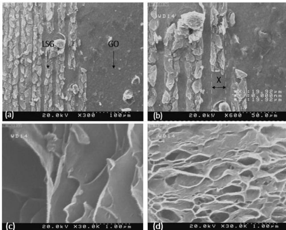
**Figure 4.** SEM images of the laser scribed surface of graphene oxide at a low (a) and a high (b) magnification. Reduction of GO and the formation of graphene sheets (c) with a clear distance between them (d).
